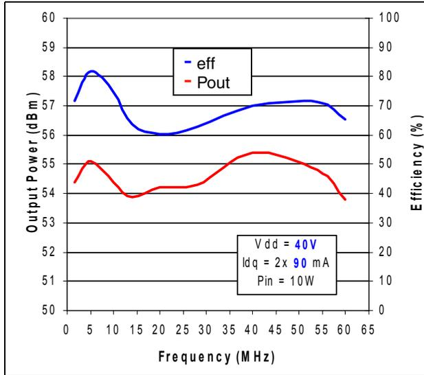
**Figure 2. Output power & efficiency vs frequency**
