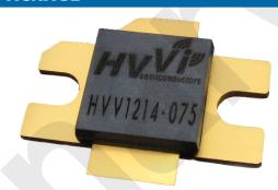
The device resides in a two-lead metal flanged package with liquid crystal polymer lid. The HV400 package style is qualified for gross leak test – MIL-STD-750D, Method 1071.6, Test Condition C.
