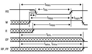
Notes: 1.  $\overline{EF}$ ,  $\overline{FF}$  and  $\overline{HF}$  may change status during reset, but flags will be valid at  $t_{RSC}$ .
