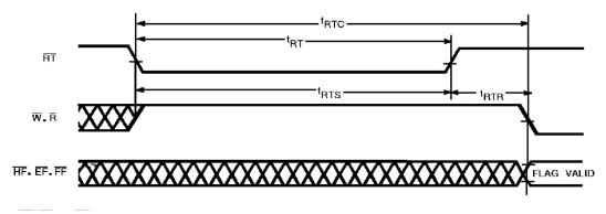
Note: 1.  $\overline{\text{EF}}$ ,  $\overline{\text{FF}}$  and  $\overline{\text{PHF}}$  may change status during Retransmit, but flags will be valid at  $t_{RTC}$
