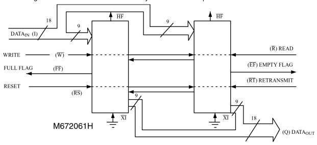
Note: Flag detection is accomplished by monitoring the  $\overline{\mathsf{FF}}$ ,  $\overline{\mathsf{EF}}$  and the  $\overline{\mathsf{HF}}$  signals on either (any) device used in the width expansion configuration. Do not connect any output control signals together.
