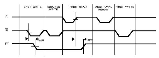
Figure 11. Empty Flag from Last Read to First Write
