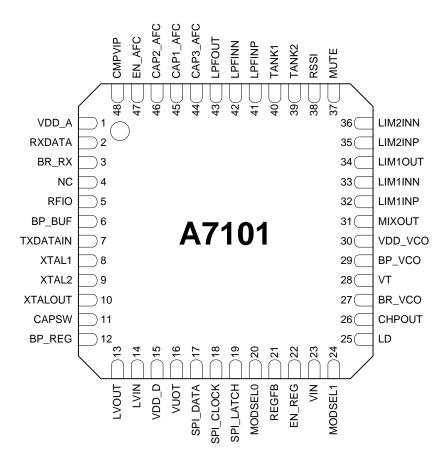
Figure 1. QFN Package Top View
