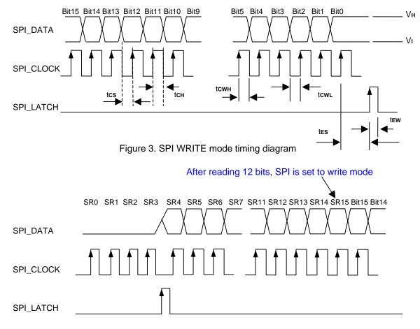
Figure 4. SPI READ mode timing diagram
