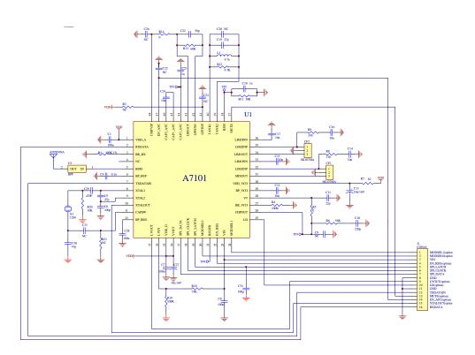
Figure 12. Application Circuit for Receiver
