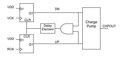
Figure 6. Phase Detector Block Diagram
