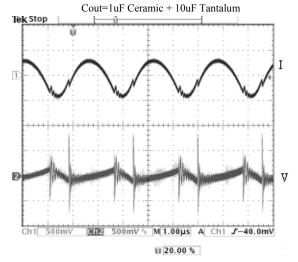
**Photo 12:** Input Reflected Ripple Voltage and Ripple Current Vin=24V, Iout = 20A with a 680uF Aluminum Electrolytic and 12uH series inductor.
