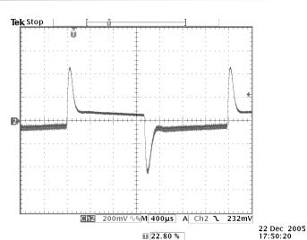
**Photo 8:** Transient Response Min Load to Max Load Vin=24V, Iout = 2 to 20A
