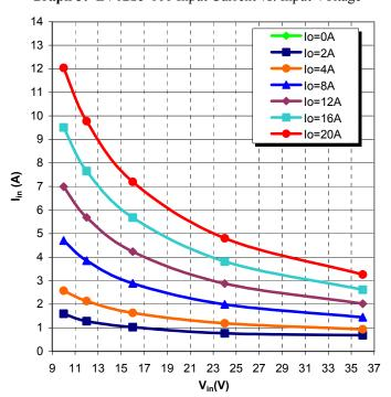
**Graph 5:** LV12S5-100 No Load Input Current and Power Dissipation vs. Input Voltage
