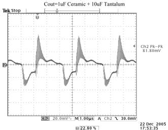
Photo 11: Output Voltage Ripple (Spike) Vin=24V, Iout = 20A Cout=1uF Ceramic + 10uF Tantalum
