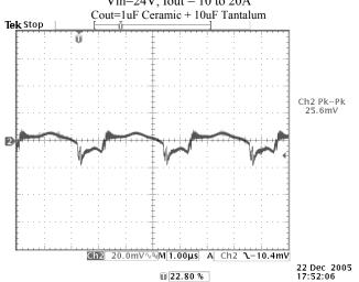
**Photo 9:** Output Voltage Ripple (20 MHz BW) Vin=24V, Iout=1.25A
