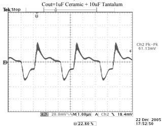
**Photo 10:** Output Voltage Ripple (20 MHz BW) Vin=24V, Jout=20A
