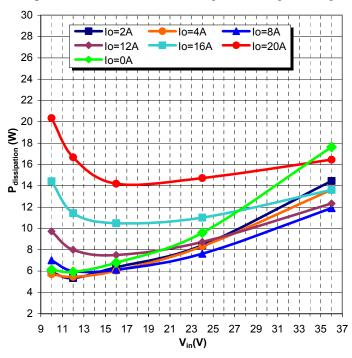
**Graph 6:** LV12S5-100 "Remote Off" Input Current and Power Dissipation vs. Input Voltage
