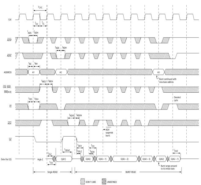
Note: 17. On this diagram, when  $\overline{CE}$  is LOW,  $\overline{CE}_1$  is LOW,  $\overline{CE}_2$  is HIGH and  $\overline{\overline{CE}}_3$  is LOW. When  $\overline{\overline{CE}}$  is HIGH,  $\overline{\overline{CE}}_1$  is HIGH or  $\overline{\overline{CE}}_2$  is LOW or  $\overline{\overline{CE}}_3$  is HIGH.
