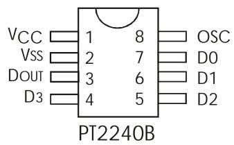
Figure 1: PT2240B Pin Configurations
