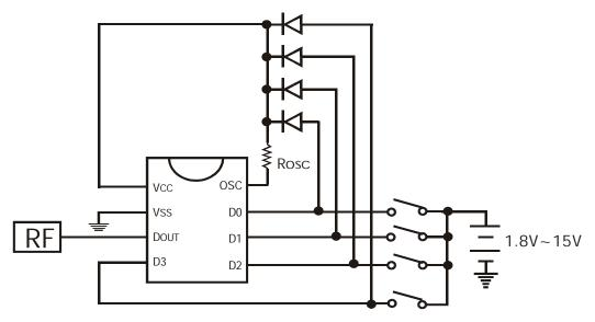
Figure 3: PT2240B Power Failure Application Circuit
