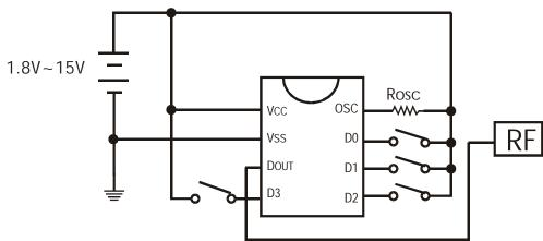
Figure 2: PT2240B (8-pin) Application Circuit
