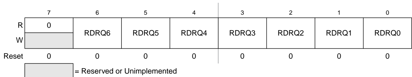
Figure 3-26. Port Q Reduced Drive Register (RDRQ)
