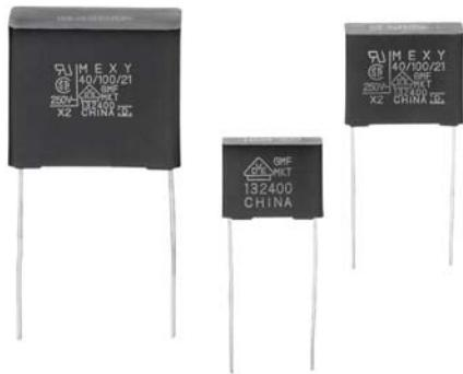
The Type MEXY metallized polyester class X2 and Y2/X2 film capacitors are ideal for across-the-line and line-to-ground interference suppression circuit applications. This product features the self-healing capabilities associated with metallized polyester, compact design and flame retardant construction meets UL 94V0.
