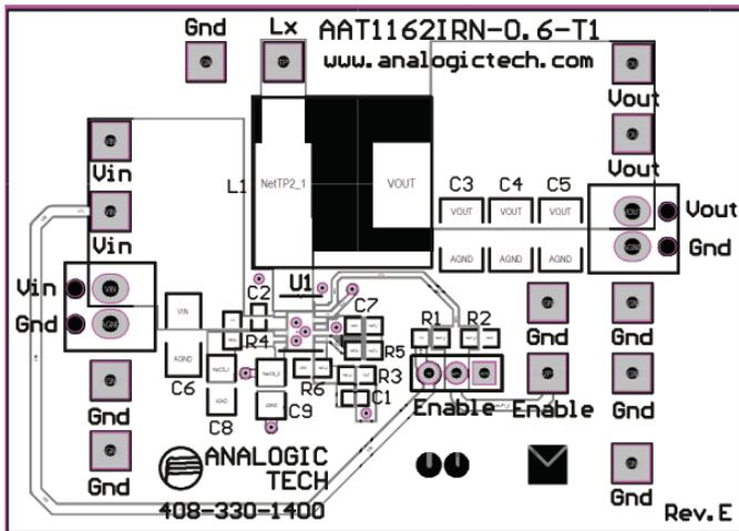
**Figure 3: AAT1162 Evaluation Board Component Side Layout.**
