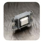
A fully screened relay offering low RF loss and high current carrying capacity, which was developed with RF design engineers in the radio communications industry. The relay coil is totally enclosed in a copper screen, resulting in lower self-heating and RF loss, and Rhodium contacts are used in the vacuum reed switches, yielding higher carry currents for a given frequency and ambient temperature.
