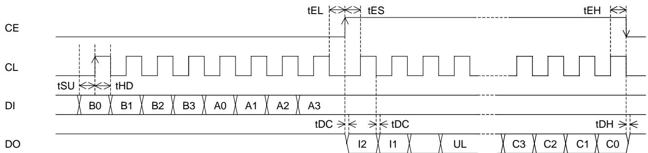
(Note) DO pin is an Nch open drain pin, so that the data varying time (tDC and tDH) differs depending on the pull-up resistance and substrate capacity.
