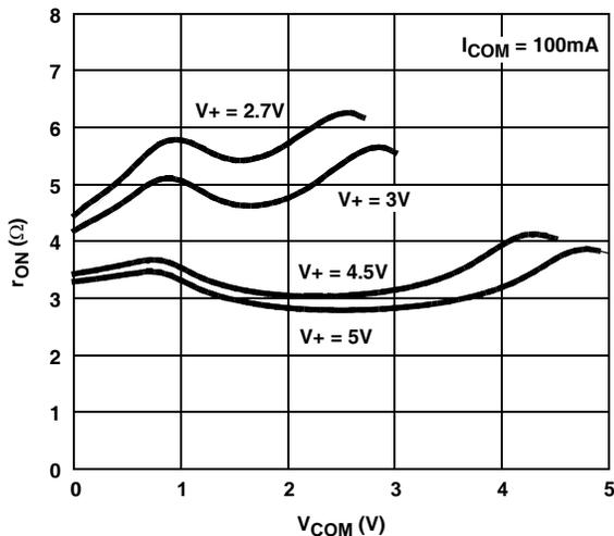
FIGURE 8. ON-RESISTANCE vs SUPPLY VOLTAGE vs SWITCH VOLTAGE
