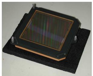
The top of the package has an optical window over the CCD active area. The CCD595 is mounted in an environmentally sealed enclosure containing the CCD array with thermoelectric coolers for controlling the operating temperature of the array.
