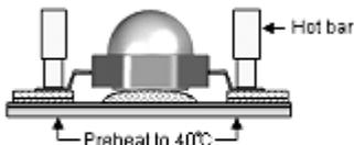
Hot bar soldering of LED emitter
