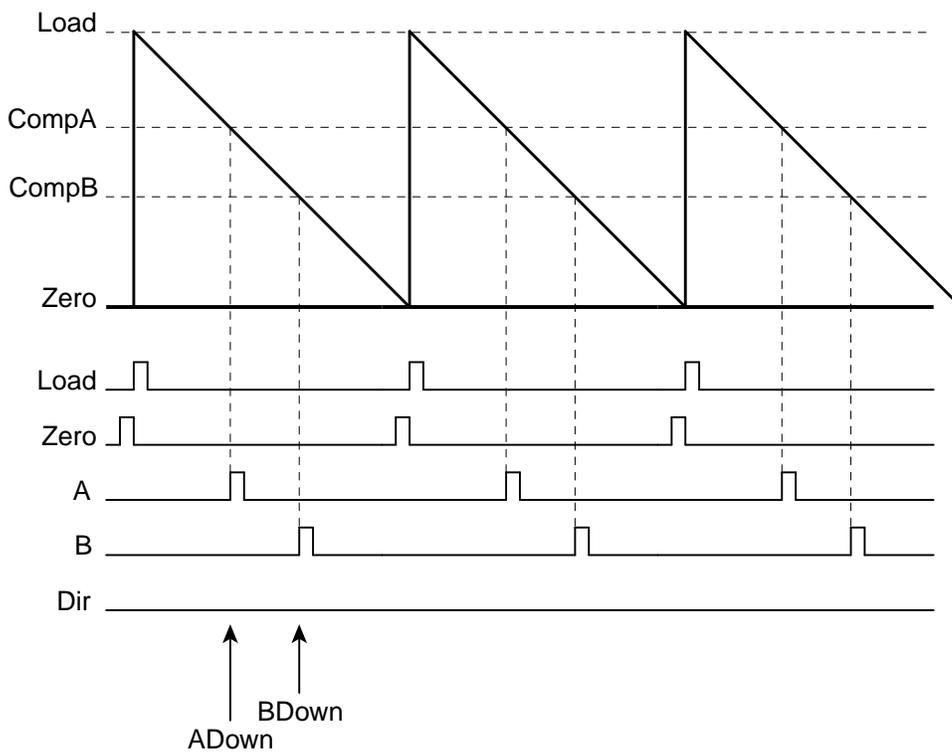
changes the duty cycle of the  $PWMA$  signal, and changing the value of comparator B changes the duty cycle of the  $PWMB$  signal.
