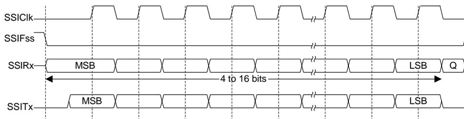
**Figure 14-5. Freescale SPI Format (Continuous Transfer) with SPO=0 and SPH=0**
