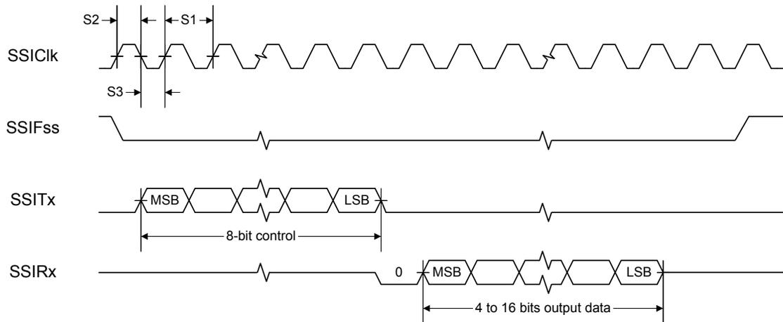
Figure 23-6. SSI Timing for SPI Frame Format (FRF=00), with SPH=1
