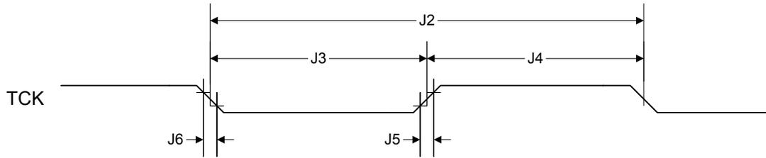
Figure 23-8. JTAG Test Access Port (TAP) Timing
