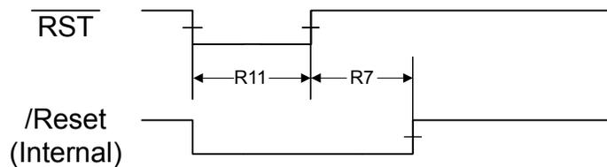
**Figure 23-11. Power-On Reset Timing**
