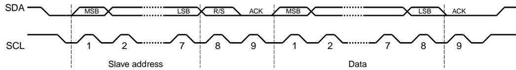
The first seven bits of the first byte make up the slave address (see Figure 15-5 on page 361). The eighth bit determines the direction of the message. A zero in the R/S position of the first byte means that the master will write (send) data to the selected slave, and a one in this position means that the master will receive data from the slave.
