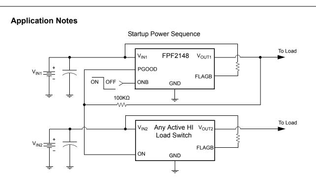
Power good function in sequential startup. No battery is loaded to the output
