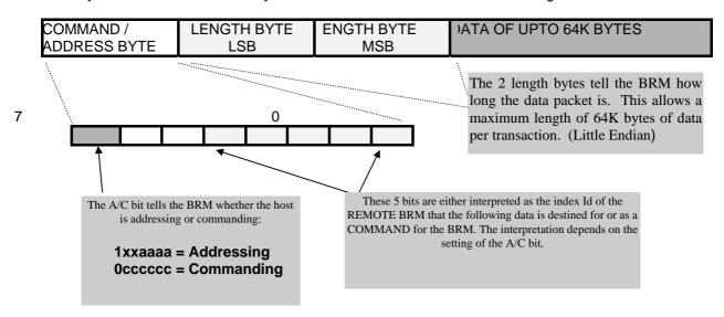
Data packets received from the HOST by the BRM are stored in a packet buffer and are transmitted to the REMOTE address automatically i.e. there is no requirement for a TX/RX line to tell the BRM to transmit. There is no requirement for the host to re-transmit data, since error correction and retransmission is handled by the BRM.
