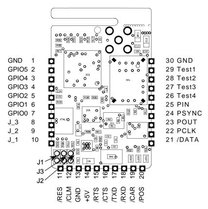
The module layout ensures that most of the common interconnects are physically co-located. For some simple applications only pins 11 to 20 are needed.
