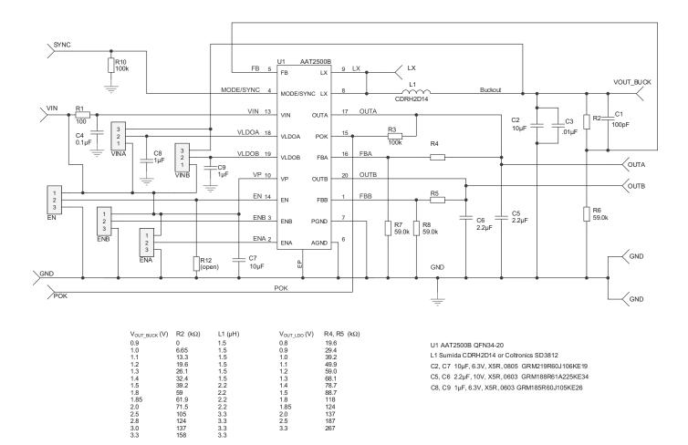
Figure 3: AAT2500B Evaluation Board Schematic.
