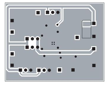
Figure 2: AAT2500B Evaluation Board Bottom Side Layout.
