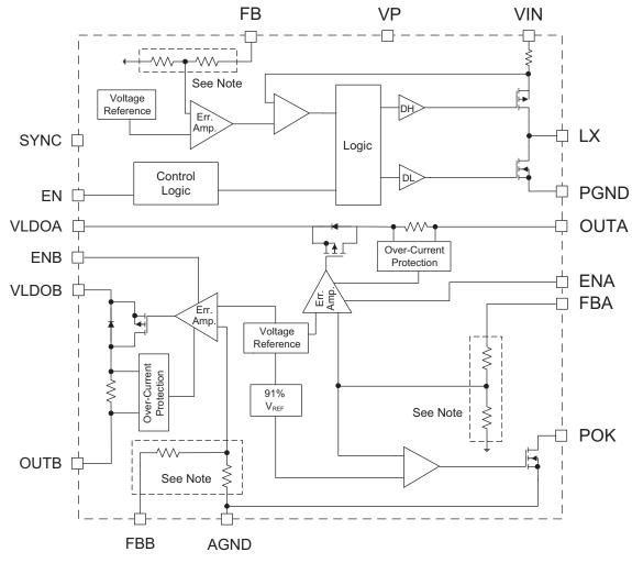
Note: For adjustable version, the internal feedback divider is omitted and the FB pin is tied directly to the internal error amplifier.
