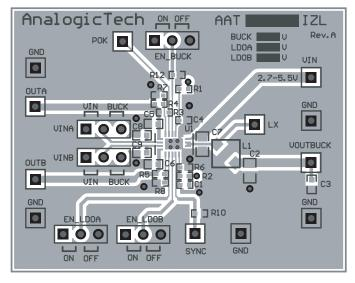
Figure 1: AAT2500B Evaluation Board Top Side Layout.
