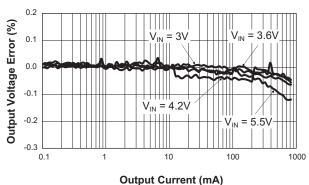
Step-Down Converter Line Regulation (V<sub>OUT</sub> = 2.5V; Forced PWM)
