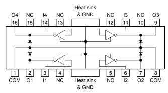
Note: The NC pins are not connected to the die. If wiring is required, it is recommended to connect the pins to the Heat sink & GND line(s).
