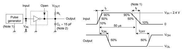
Note 1: Pulse Width 50  $\mu s,$  Duty Cycle 10% Output Impedance 50  $\Omega,$   $t_{r}$   $\leq$  5 ns,  $t_{f}$   $\leq$  10 ns
