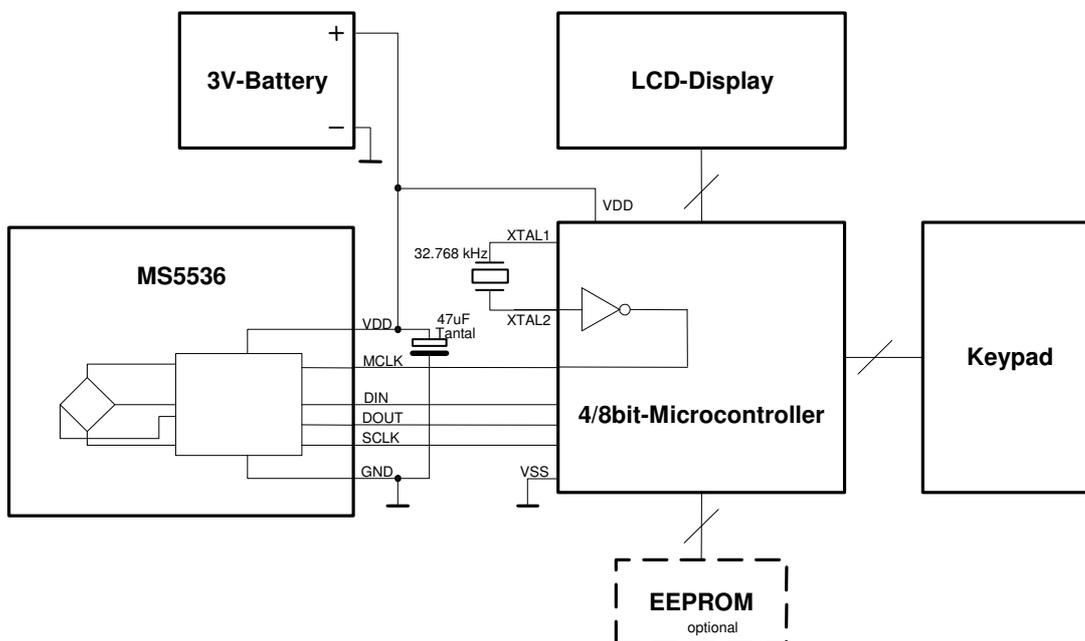
Fig. 7: Application example of the MS5536 for a battery powered device
