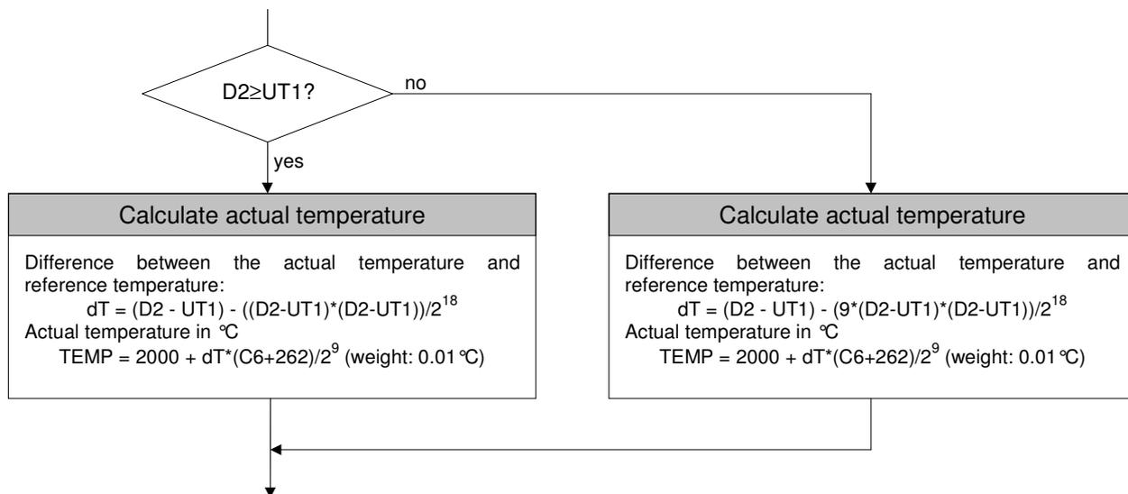
Fig. 5: Flow chart for calculating the temperature to the optimum accuracy. The value for  $dT$  thus obtained is then used for the calculation of the temperature compensated pressure as shown in Fig. 3.
