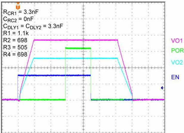
An alternative method here shows an example of a  $V_{DDQ}$  &  $V_{TT}$  solution for a DDR memory power supply. Note that POR is taken from Vo1 as  $POR_2$  will not go high. This is because POR is set high when  $FB > 0.9 \cdot V_{REF}$ . In this example,  $FB_2$  is regulated to  $\frac{1}{2} \cdot V_{REF}$ .
