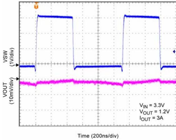
**Switch Node / Output Voltage**
