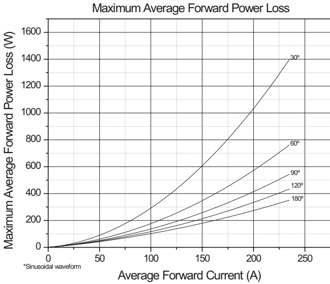
Fig. 3 - Forward Power Loss Characteristics
