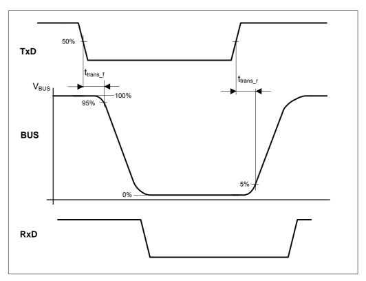
Figure 2 - Transmit delay
