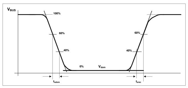
Figure 7 - Slope time and slew rate calculation in accordance to LIN 1.3
