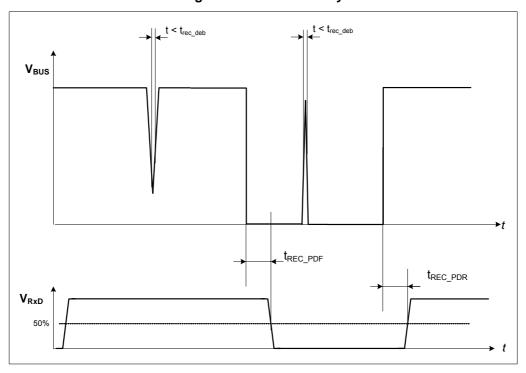
Figure 3 – Receiver debouncing and propagation delay
