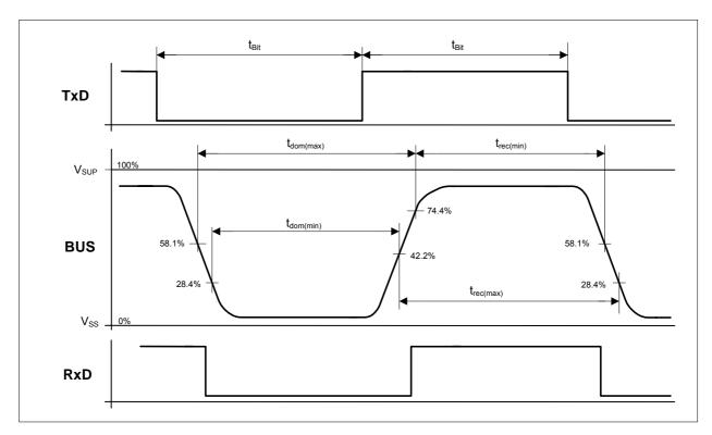
Figure 8 - Duty cycle calculation in accordance to LIN 2.0
