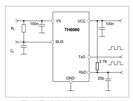
Figure 4 - Test circuit for dynamic characteristics
