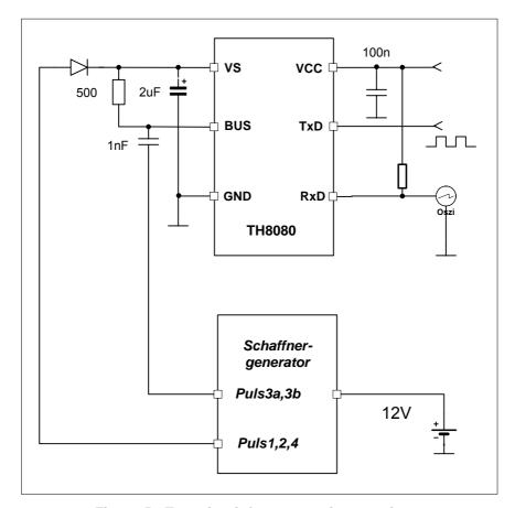
Figure 5 - Test circuit for automotive transients
