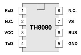
Figure 10 - Pin description SOIC8 package
