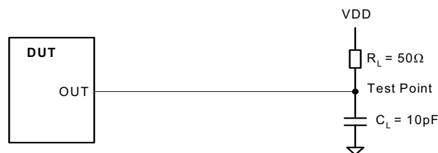
Figure 19. Load Circuit - High to Low Slew Measurement
