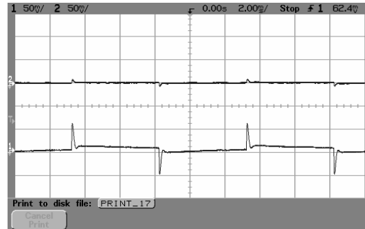
ALQ07FM 50%-75%-50% I_{o1,nom} ( I_{o1} ) load change, I_{o2} = 50\%I_{o2,nom} (ch1: V_{o1} ,ch2: V_{o2} )
