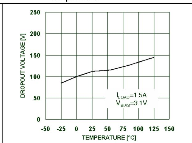
Figure 13. Dropout voltage ( $V_{IN}-V_{OUT}$ ) vs temperature
