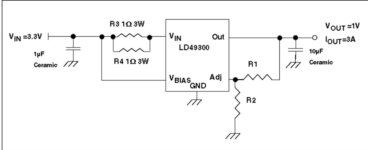
Figure 4. LD49300 plus DC/DC pre-regulator to reduce power dissipation
