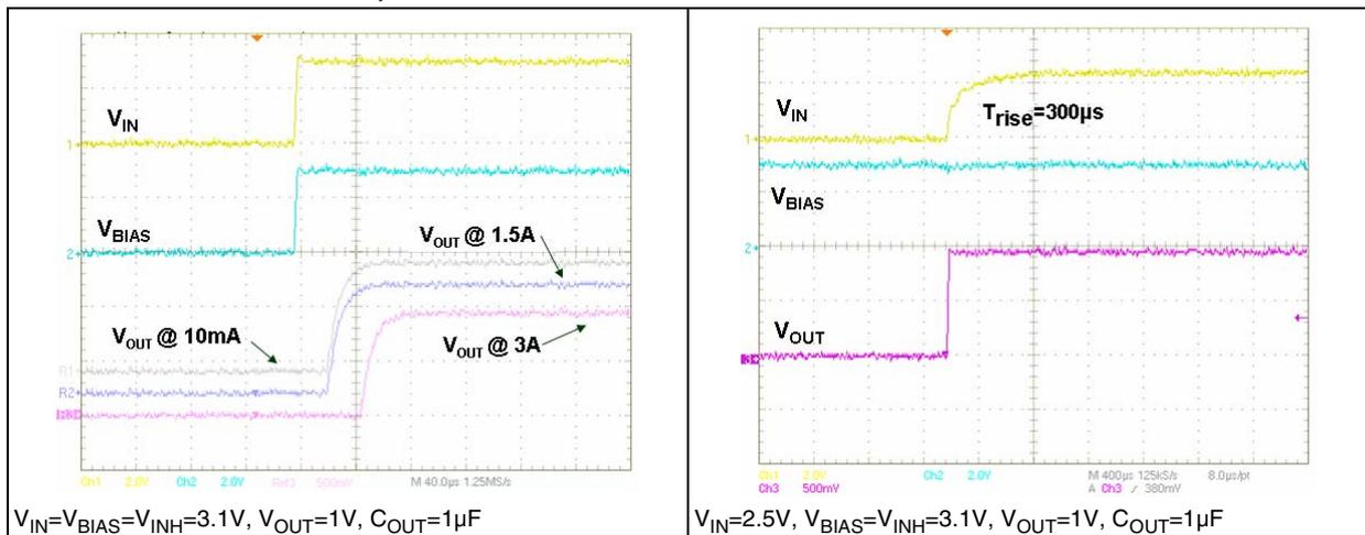
**Figure 23.  $V_{IN}$  Start Up transient response ( $V_{BIAS}$  Start Up before  $V_{IN}$ )**
