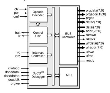
Interrupt Controller - DF6811CPU has implemented only an external interrupts from pins IRQ and XIRQ. The interrupts are activated at low level (XIRQ,IRQ pins) or falling edge (IRQ pin) and are sampled each 1 system clock at the rising edge of CLK.
