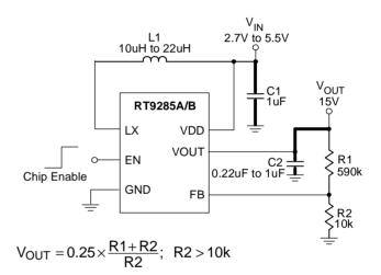
Figure 5. Application for Constant Output Voltage
