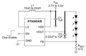
Figure 3. Application for Driving 4 Series WLEDs
