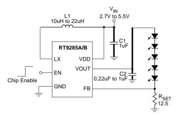
Figure 4. Application for Driving 5 Series WLEDs
