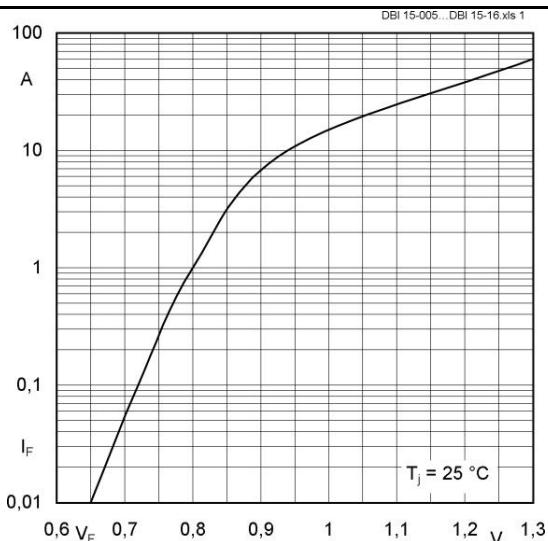
Fig. 1 : Forward characteristic (typical values)
