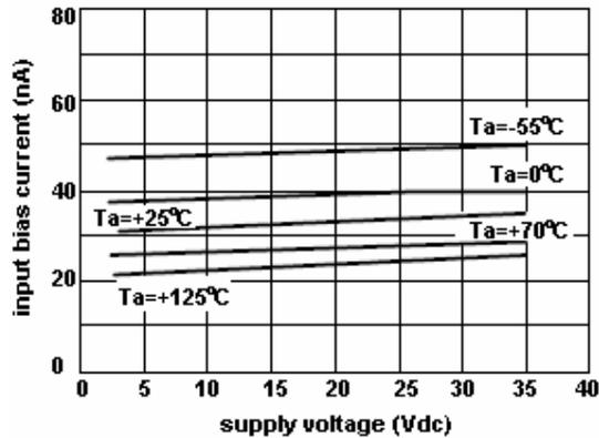
Figure 1. input bias current vs power supply voltage
