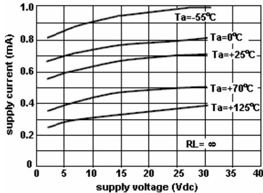
Figure 3. power supply current vs power supply voltage
