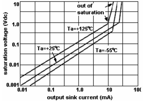
Figure 2. output saturation voltage vs output sink current
