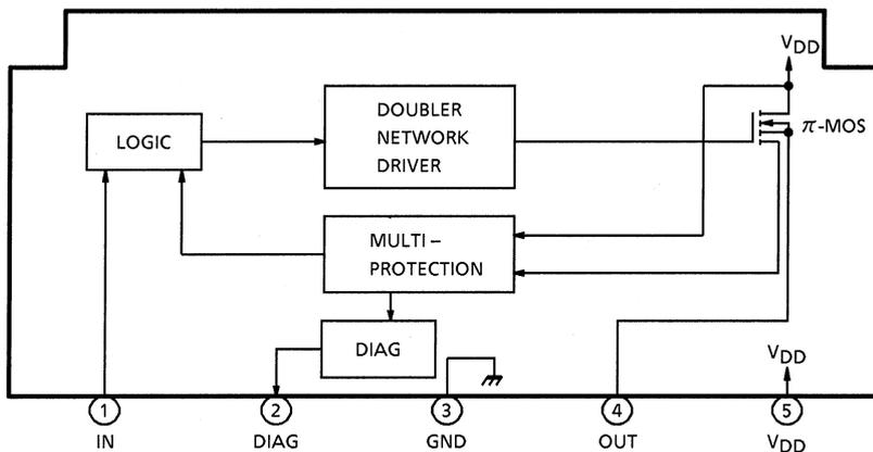
Note: Due to its MOS structure, this product is sensitive to static electricity.
