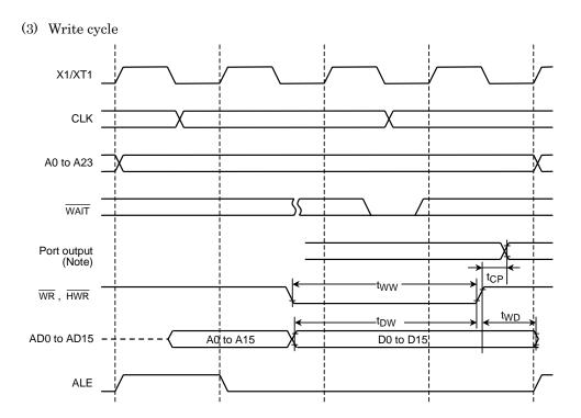
Note: Since the CPU accesses the internal area to write data to a port, the control signals of external pins such as  $\overline{\text{WR}}$  and  $\overline{\text{CS}}$  are not enabled. Therefore, the above waveform diagram should be regarded as depicting internal operation. Please also note that the timing and AC characteristics of port input/output shown above are typical representation. For details, contact your local Toshiba sales representative.
