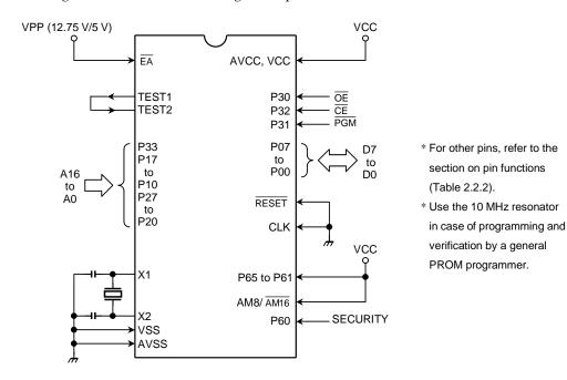
Figure 3.2.1 shows the setting of the pins in PROM mode.
