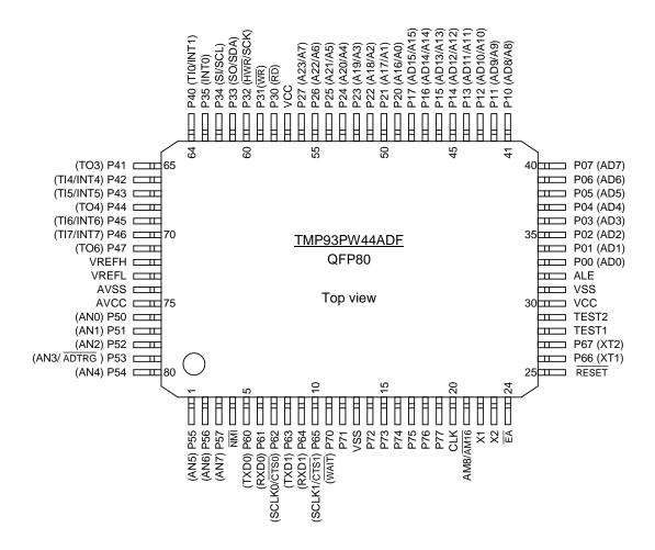
Figure 2.1.1 Pin Assignment (P-QFP80-1420-0.80B)
