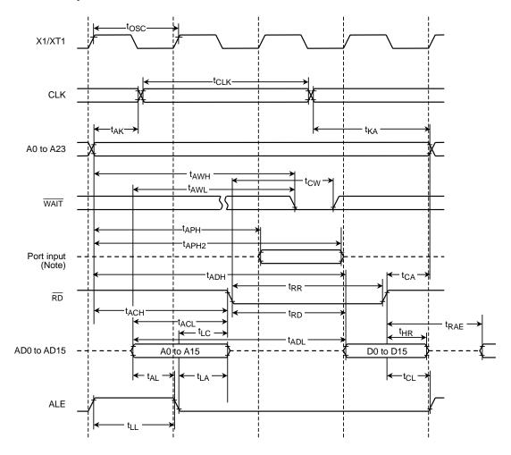
Note: Since the CPU accesses the internal area to read data from a port, the control signals of external pins such as  $\overline{\text{RD}}$  and  $\overline{\text{CS}}$  are not enabled. Therefore, the above waveform diagram should be regarded as depicting internal operation. Please also note that the timing and AC characteristics of port input/output shown above are typical representation. For details, contact your local Toshiba sales representative.
