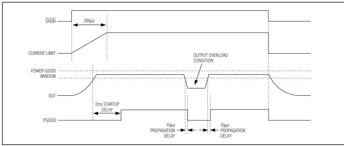
Figure 3. MAX8794 PGOOD and Soft-Start Waveforms
