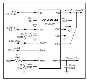
Figure 1. Standard Application Circuit
