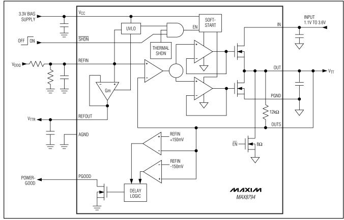
Figure 2. Functional Diagram
