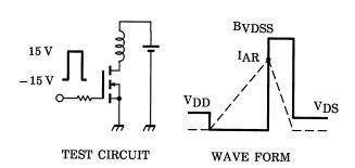
$$\begin{aligned} R_G &= 25~\Omega \\ V_{DD} &= 50~V,~L = 1.48~mH \end{aligned} \qquad EAS = \frac{1}{2} \cdot L \cdot I^2 \cdot \left( \frac{BVDSS}{BVDSS - VDD} \right) \end{aligned}$$
