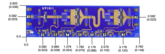
Units: millimeters (inches) Bond pad dimensions are shown to center of bond pad. Thickness: 0.110 +/- 0.010 (0.0043 +/- 0.0004), Backside is ground, Bond Pad/Backside Metallization: Gold All Bond Pads are 0.100 x 0.100 (0.004 x 0.004). Bond pad centers are approximately 0.109 (0.004) from the edge of the chip. Dicing tolerance: +/- 0.005 (+/- 0.0002). Approximate weight: 2.145 mg.
