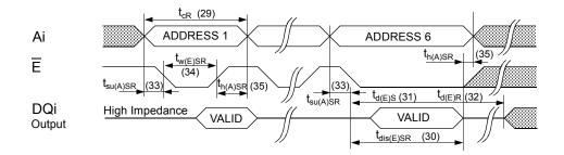
v: E must be used to clock in the address sequence for the Software controlled STORE and RECALL cycles.
