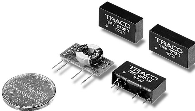
The TMV-EN series are dc/dc converters with supplementary high I/O-isolation, to comply with safety standard IEC/EN 60950. They are designed for applications where approved isolation is required, i.e. information technology equipment or medical equipment. SMT-design and a special transformer technology made it possible to build these converters in a very small SIP-package, requiring a minimum space on the PCB.
