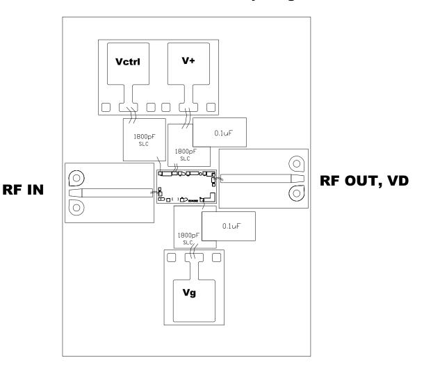
Note: Input and Output ports are DC coupled.
