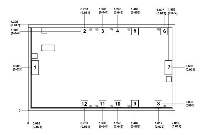
Units: millimeters (inches) Thickness: 0.100 (0.004)
