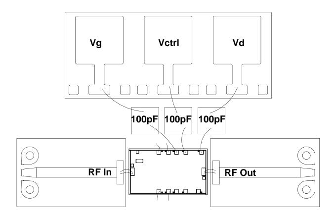
All DC connections may be brought in from either side of the chip (Use Pad 4 or 10, Pad 5 or 9, and Pad 6 or 8) 0.01uF external Caps are recommended on Drain, Gate line, 10 ohm external series R between 100pF cap and 0.01uF cap is recommended for Gate line Source connections (Pad 2, 3, 11, 12) are bonded to ground
