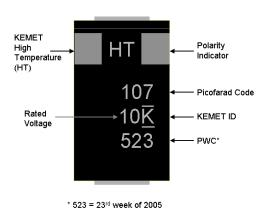
Figure 3. Component marking diagram for T498 capacitor.
