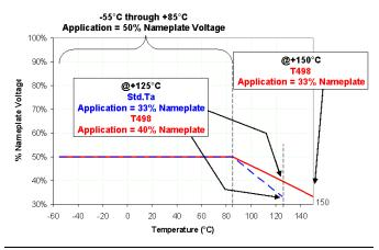
Figure 5. Recommended application voltages versus temperature.
