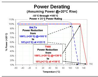
Figure 6. Power derating to maximum temperatures.
