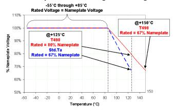
Figure 4. Voltage-temperature derating for standard and T498 capacitors.
