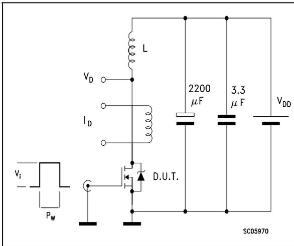
Figure 16: Switching Times Test Circuit For Resistive Load
