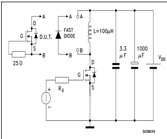
Figure 18: Unclamped Inductive Waferform
