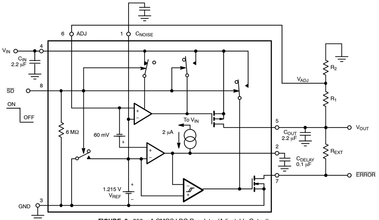
**FIGURE 6.** 350-mA CMOS LDO Regulator (Adjustable Output)
