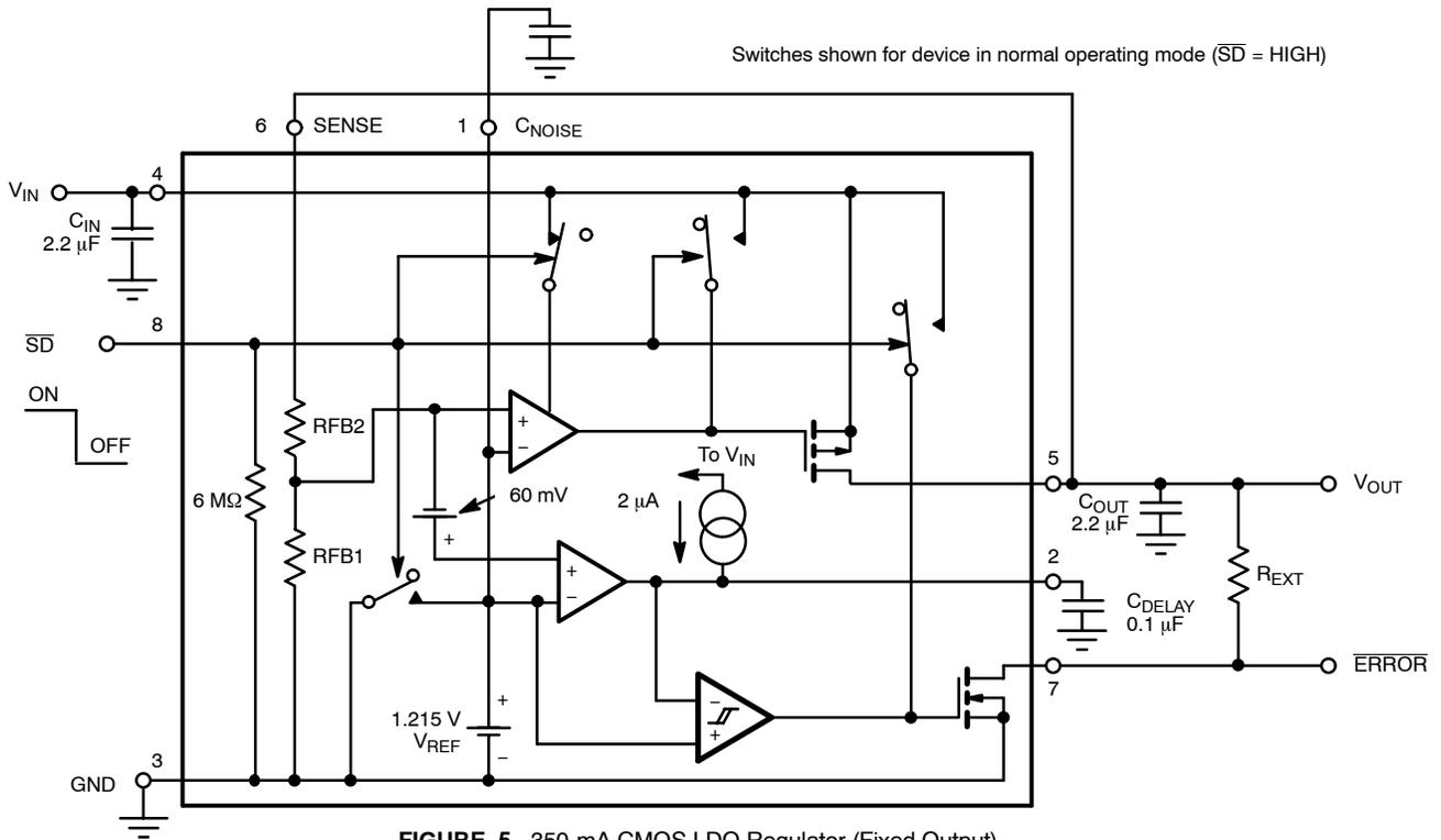
**FIGURE 5.** 350-mA CMOS LDO Regulator (Fixed Output)
