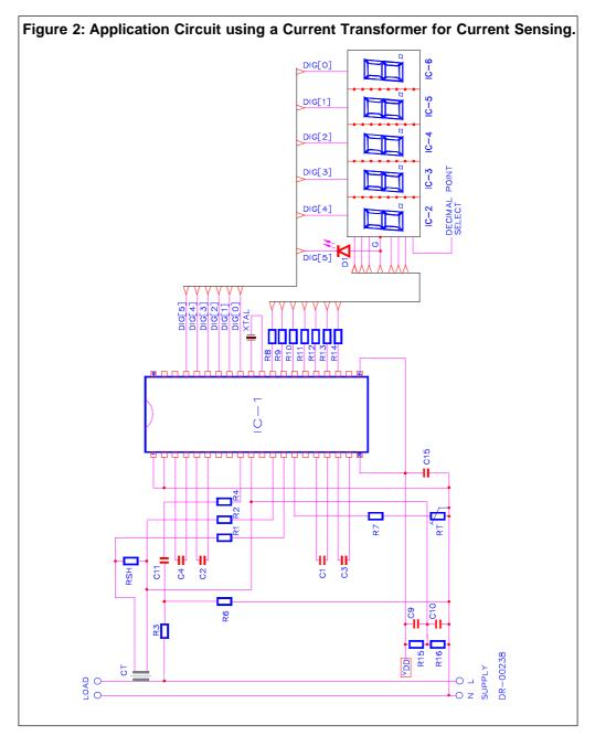
Note: Capacitor C11 may be selected for phase compensation and DC blocking.
