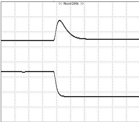
**Figure 7:** Output voltage response to step-change in load current (100%-50% of  $I_o$ , max;  $di/dt = 1A/\mu s$ ). Load cap: 10 $\mu F$ , 100 m $\Omega$ ESR tantalum capacitor and 1 $\mu F$  ceramic capacitor. Top Trace: Vout (50mV/div, 100 us/div), Bottom Trace: Iout (2.42A/div).
