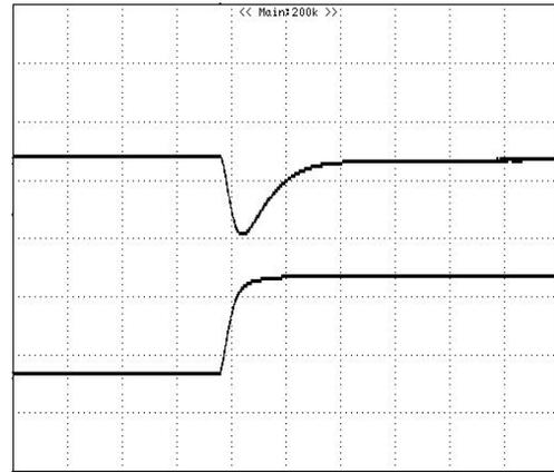
**Figure 6:** Output voltage response to step-change in load current (50%-100% of  $I_o$ , max;  $di/dt = 1A/\mu s$ ). Load cap: 10 $\mu F$ , 100 m $\Omega$  ESR tantalum capacitor and 1 $\mu F$  ceramic capacitor. Top Trace: Vout (50mV/div, 100 us/div), Bottom Trace: Iout (2.42A/div).
