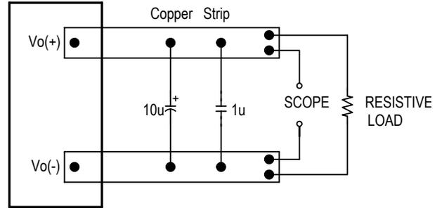
**Figure 10:** Output voltage noise and ripple measurement test setup. Scope measurement should be made using a BNC cable (length shorter than 20 inches). Position the load between 51 mm to 76 mm (2 inches to 3 inches) from the module.
