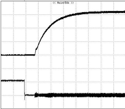
**Figure 5:** Turn-on transient at zero load current (Constant resistance mode) (1 ms/div). **Vin:** 48V; Top Trace: Vout (1V/div); Bottom Trace: ON/OFF Control (5V/div).
