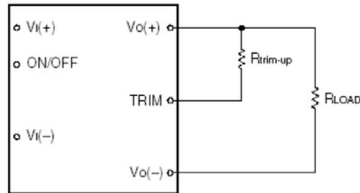
**Figure 16:** Circuit configuration for trim-up (increase output voltage)
