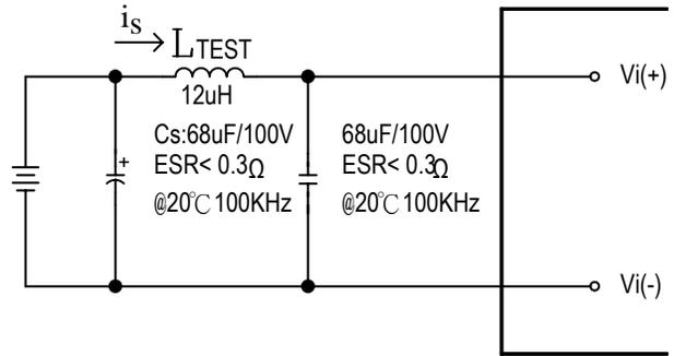
**Figure 8:** Test set-up diagram showing measurement points for Input Reflected Ripple Current (Figure 9). Note: Measured input reflected-ripple current with a simulated source Inductance ( $L_{TEST}$ ) of 12  $\mu H$ . Capacitor  $C_s$  offset possible battery impedance.
