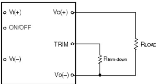
**Figure 15:** Circuit configuration for trim-down (decrease output voltage)
