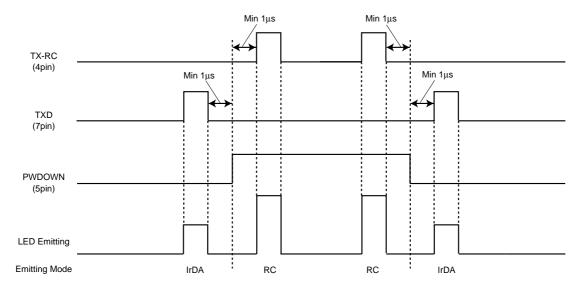
$* If TX-RC \ or \ TXD \ input \ pulse \ width \ is \ wider \ than \ 48\mu s, \ output \ LED \ emitting \ pulse \ will \ be \ turn \ off \ approximately \ 48\mu s.$
