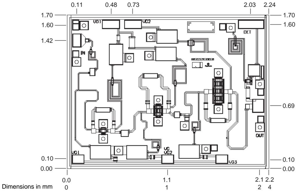
Chip Size is 2.24mm x 1.70mm X 100µm. Back of chip is RF and DC Ground.
