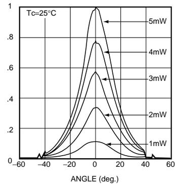
Fig.4 Perpendicular for field pattern
