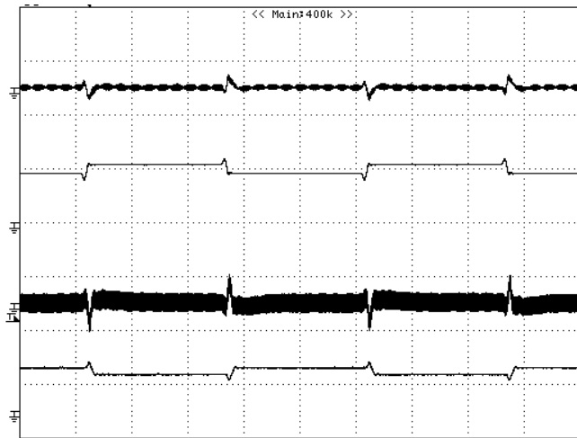
Figure 15: Output voltage response to step-change in load current Iout2 and Iout1 (75%-50%-75% of Io, max; di/dt = 2.5A/μs). Load cap: 470μF, 35mΩ ESR solid electrolytic capacitor and 1μF ceramic capacitor. Ch1=Vout1 (100mV/div), Ch2=Iout1 (5A/div), Ch3=Vout2 (100mV/div), Ch4=Iout2 (5A/div) Scope measurement should be made using a BNC cable (length shorter than 20 inches). Position the load between 51 mm to 76 mm (2 inches to 3 inches) from the module.
