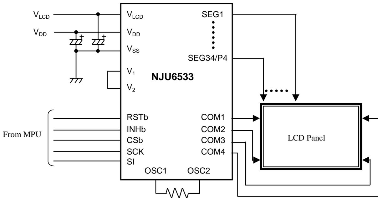
Note) Because display data is not yet stable just after  $V_{DD}$  on, if LCD panel is turned on, unexpected pattern will be displayed, therefore, keep INHb terminal to "L" level until data transfer from MPU is over.
